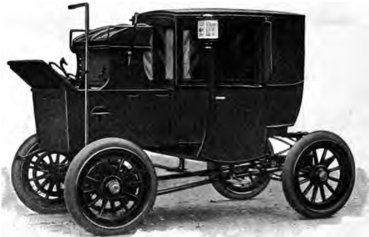
FIG. 59.—Front-Driving Brougham of the Electric Vehicle Co., used in New York City. This model, which is no longer manufactured, represents a construction very suitable for city service, but quite inappropriate for country and general use.
